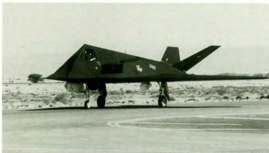
Lockheed constructed the F-117A using proven technologies from other aircraft. For example, the INS is adapted from the B-52, and the flight controls are those of the F-16.
