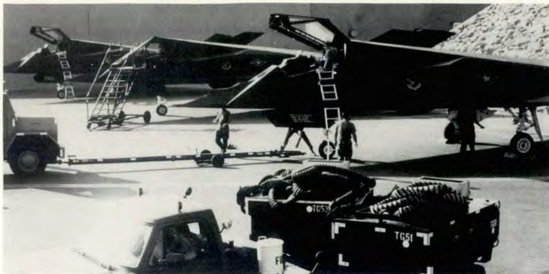
TSgt Paddock explains F-117A maintenance as "slightly more difficult than on the F-15 and F-16 because all parts are located up inside the aircraft."
